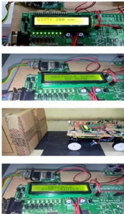
Fig 2. Output of the ultrasonic sensor used in the project
