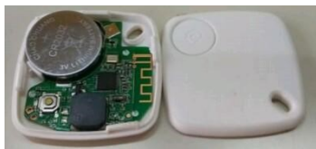
Fig 12. Anti-theft lost device work as BLE tags.[16]
