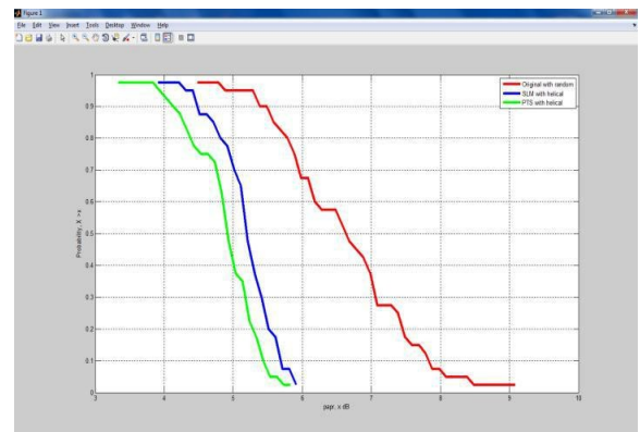
Fig 8. Comparison of PAPR reduction performance between SLM and PTS algorithm for helical interleaved OFDM
