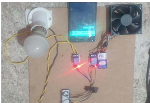
Fig 2. Light and fan control system
