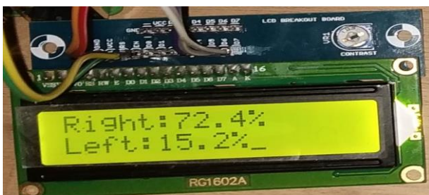
Fig 4. Density displayed on LCD display
