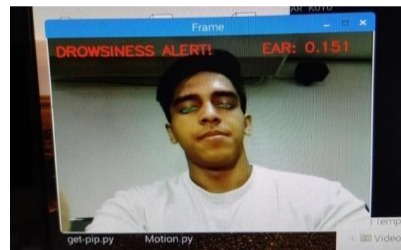
Fig 8. The EAR value before closing the eyelids
