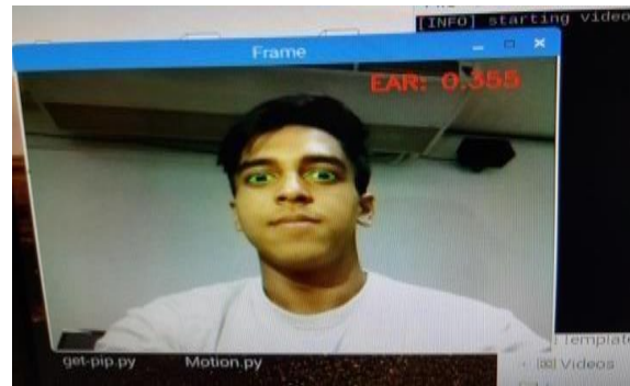
Fig 6. The EAR value before closing the eyelids
