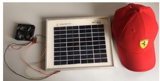
Fig 4. Solar power cap design components
