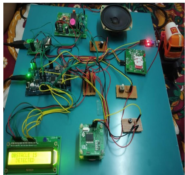
Fig 2. Obstacle detection using IR Sensor
