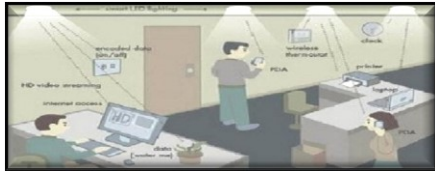
Fig 2. LiFi system connecting devices in a room
