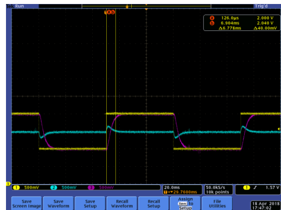
Fig 5. Plant output with Controller of Spool loop
