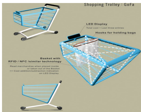
Fig 8. RFID reader working inside the trolley.
